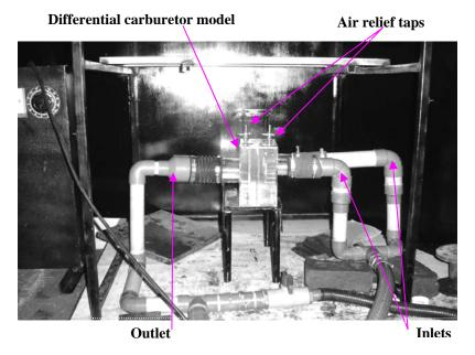
Plate 2 Flow visualization study inside the carburetor model
