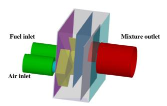
Figure 1: 3D-Model of Producer gas carburetor
