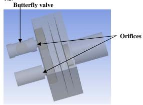
Figure 2: Geometric model of Producer Gas carburetor
