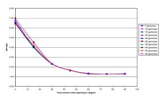
Figure 8 Air Fuel Characteristic curve for different fuel inlet valve opening derived from CFD Analysis
