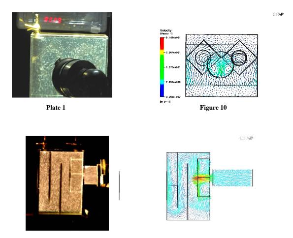
Figure 11: Comparison of flow between experimental and computational results
