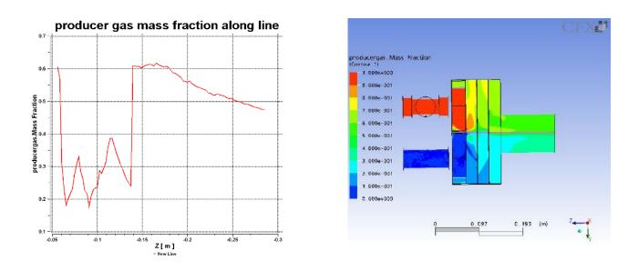
Figure 9 Producer gas Mass fraction on a line for mixture flow rate of 25g/s and for 90 degree butterfly valve opening.
