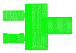
Figure 4: Mesh Geometry Model of Producer Gas Carburetor
