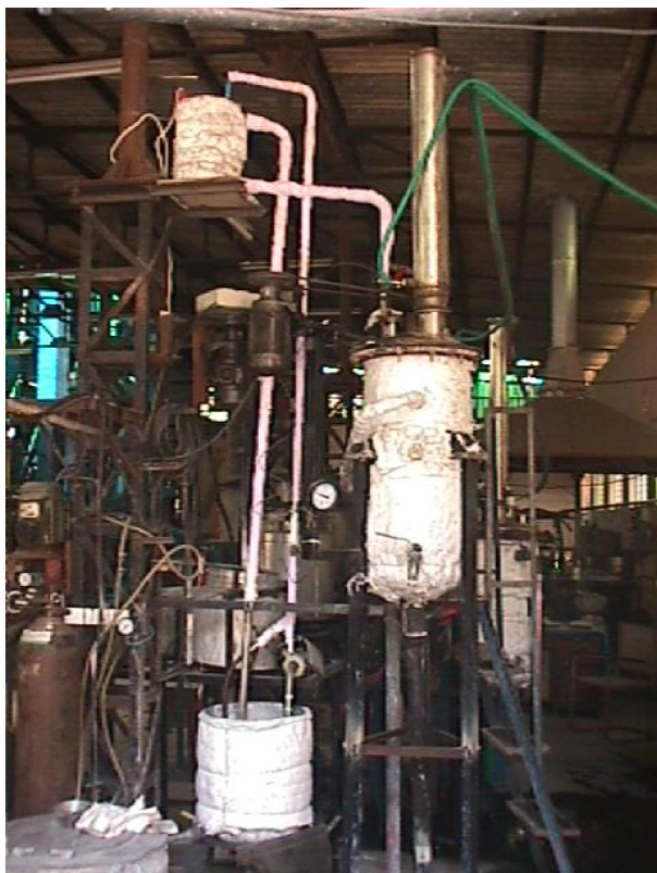
Plate 6.3 Precipitator used for Silica Production
