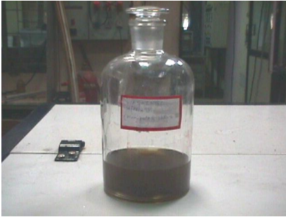
Washing from Intake Manifold and Butterfly Valve
