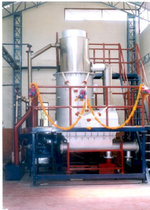
75 kg/hr gasifier system at NIE, Mysore
