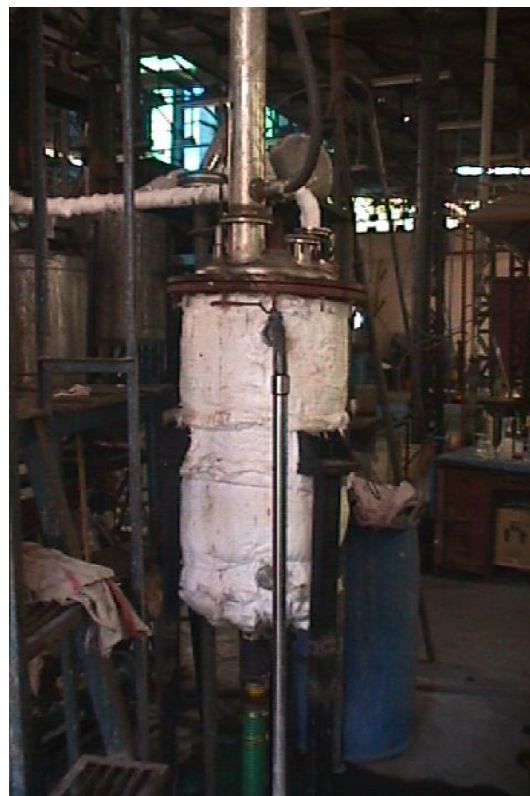
Plate 6.4 Digester for ash silica extraction from ash
