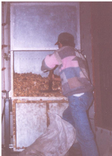
Plate 2.6 Drier using engine exhaust heat
